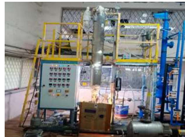
Pilot scale reactor/pyrolyser (Haste- alloy reactor tube with electrical heating and scrubber)
